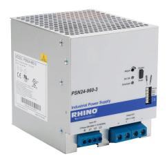
RHINO PRO PSN series switching power supply, 24 VDC @ 40A/960W (adjustable), 480 VAC nominal input, 3-phase, enclosed, aluminum housing, 35mm DIN rail mount, screw terminals.
