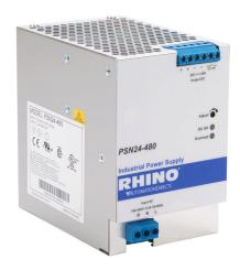
RHINO PRO PSN series switching power supply, 24 VDC @ 20A/480W (adjustable), 120/240 VAC or 110-300VDC nominal input, 1-phase, enclosed, aluminum housing, 35mm DIN rail mount, screw terminals.
