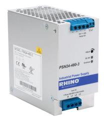
RHINO PRO PSN series switching power supply, 24 VDC @ 20A/480W (adjustable), 480 VAC nominal input, 3-phase, enclosed, aluminum housing, 35mm DIN rail mount, screw terminals.
