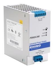
RHINO PRO PSN series switching power supply, 24 VDC @ 10A/240W (adjustable), 120/240 VAC or 110-300VDC nominal input, 1-phase, enclosed, aluminum housing, 35mm DIN rail mount, screw terminals.
