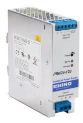
RHINO PRO PSN series switching power supply, 24 VDC @ 5A/120W (adjustable), 120/240 VAC or 110-300VDC nominal input, 1-phase, enclosed, aluminum housing, 35mm DIN rail mount, screw terminals.
