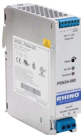
RHINO PRO PSN series switching power supply, 24 VDC @ 3.4A/81.6W (adjustable), 120/240 VAC or 110-300VDC nominal input, 1-phase, enclosed, aluminum housing, 35mm DIN rail mount, screw terminals.
