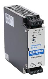
RHINO redundancy module, 2 inputs, 24 VDC nominal input, 24-27 VDC output, 15A, alarm contact for operation monitoring, active current sharing, removable screw terminals. Requires (2) PSM24 power supplies.
