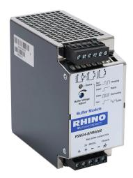
RHINO buffer module, 1 input, 24 VDC nominal input, 22-28 VDC output, 25A, potentiometer, alarm contact for operation monitoring, removable screw terminals. Requires 24 VDC power supply.
