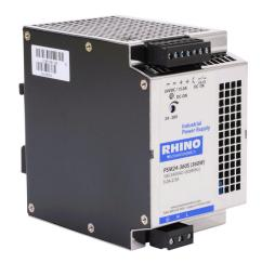
RHINO SELECT PSM series switching power supply, 24 VDC @ 15A/360W (adjustable), 120/240 VAC nominal input, 1-phase, enclosed, metal housing, 35mm DIN rail mount, removable screw terminal.
