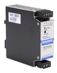
RHINO SELECT PSM series switching power supply, 24 VDC @ 3.75A/90W (adjustable), 120/240 VAC nominal input, 1-phase, enclosed, metal housing, 35mm DIN rail mount, removable screw terminal.
