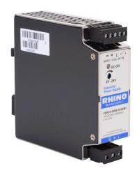
RHINO SELECT PSM series switching power supply, 24 VDC @ 3.75A/90W (adjustable), 120/240 VAC nominal input, 1-phase, enclosed, metal housing, 35mm DIN rail mount, removable screw terminal, NEC Class 2.
