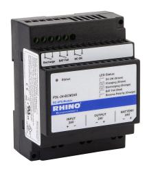
RHINO battery control module, 1 input, 24 VDC nominal input, 23-28 VDC output, 10A, alarm contact for operation monitoring, screw terminals. Requires power supply, 24V battery (usersupplied).
