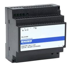
RHINO PSL series switching power supply, 24 VDC @ 3.8A/91.2W (adjustable), 120/240 VAC or 125-250 VDC nominal input, 1-phase, enclosed, plastic housing, 35mm DIN rail mount, screw terminals, NEC Class 2.
