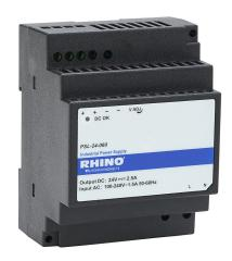
RHINO PSL series switching power supply, 24 VDC @ 2.5A/60W (adjustable), 120/240 VAC or 125-375 VDC nominal input, 1-phase, enclosed, plastic housing, 35mm DIN rail mount, screw terminals, NEC Class 2.
