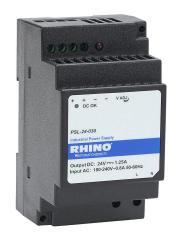
RHINO PSL series switching power supply, 24 VDC @ 1.25A/30W (adjustable), 120/240 VAC or 125-375 VDC nominal input, 1-phase, enclosed, plastic housing, 35mm DIN rail mount, screw terminals, NEC Class 2.
