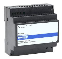
RHINO PSL series switching power supply, 12 VDC @ 6A/72W (adjustable), 120/240 VAC or 125-375 VDC nominal input, 1-phase, enclosed, plastic housing, 35mm DIN rail mount, screw terminals.
