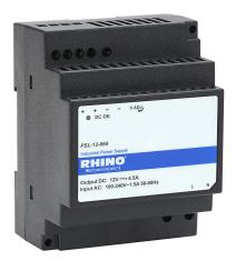
RHINO PSL series switching power supply, 12 VDC @ 4.5A/54W (adjustable), 120/240 VAC or 125-375 VDC nominal input, 1-phase, enclosed, plastic housing, 35mm DIN rail mount, screw terminals, NEC Class 2.
