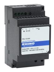
RHINO PSL series switching power supply, 12 VDC @ 2.1A/25W (adjustable), 120/240 VAC or 125-375 VDC nominal input, 1-phase, enclosed, plastic housing, 35mm DIN rail mount, screw terminals, NEC Class 2.
