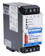
RHINO battery control module, 2 inputs, 24/48 VDC nominal input, 23-27 VDC / 47-55 VDC output, 15A at 24 VDC, 7.5A at 48 VDC, alarm contact for operation monitoring, screw terminals. Requires power supply, 12V battery (user-supplied).
