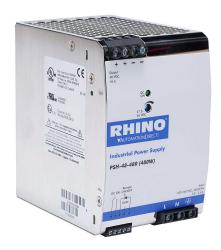
RHINO PRO PSH series switching power supply, 48 VDC @ 10A/480W (adjustable), 120/240 VAC nominal input, 1-phase, enclosed, metal housing, 35mm DIN rail mount, screw terminals, hazardous location rated.
