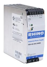
RHINO PRO PSH series switching power supply, 48 VDC @ 5A/240W (adjustable), 120/240 VAC nominal input, 1-phase, enclosed, metal housing, 35mm DIN rail mount, screw terminals, hazardous location rated.
