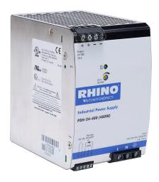
RHINO PRO PSH series switching power supply, 24 VDC @ 20A/480W (adjustable), 120/240 VAC nominal input, 1-phase, enclosed, metal housing, 35mm DIN rail mount, screw terminals, hazardous location rated.
