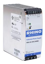
RHINO PRO PSH series switching power supply, 24 VDC @ 10A/240W (adjustable), 120/240 VAC nominal input, 1-phase, enclosed, metal housing, 35mm DIN rail mount, screw terminals, hazardous location rated.
