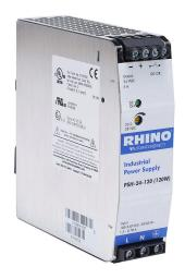
RHINO PRO PSH series switching power supply, 24 VDC @ 5A/120W (adjustable), 120/240 VAC nominal input, 1-phase, enclosed, metal housing, 35mm DIN rail mount, screw terminals, hazardous location rated.
