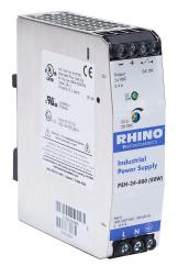
RHINO PRO PSH series switching power supply, 24 VDC @ 3.4A/80W (adjustable), 120/240 VAC nominal input, 1-phase, enclosed, metal housing, 35mm DIN rail mount, screw terminals, hazardous location rated.
