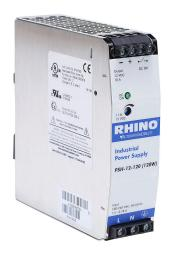
RHINO PRO PSH series switching power supply, 12 VDC @ 10A/120W (adjustable), 120/240 VAC nominal input, 1-phase, enclosed, metal housing, 35mm DIN rail mount, screw terminals, hazardous location rated.
