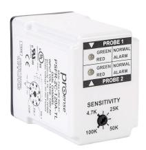
ProSense pump seal failure relay, socket mount, finger-safe, 120 VAC coil voltage, SPST, (1) N.O., 5A contact rating, 8-pin, LED indicator(s), dual channel for (2) pump monitoring. Relay becomes UL listed when used with 70169-D relay socket.
