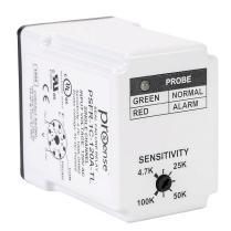
ProSense pump seal failure relay, socket mount, finger-safe, 120 VAC coil voltage, SPDT, (1) N.O., (1) N.C., 10A contact rating, 8-pin, LED indicator(s), single channel for (1) pump monitoring. Relay becomes UL listed when used with 70169-D relay socket.
