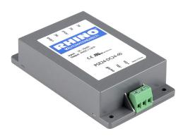
RHINO DC to DC converter, 18-75 VDC input, 24 VDC output, 1.67A, 40W, plastic housing, encapsulated, chassis mount, screw terminal.
