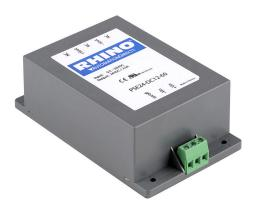
RHINO DC to DC converter, 9.5-36 VDC input, 24 VDC output, 2.5A, 60W, plastic housing, encapsulated, chassis mount, screw terminal.
