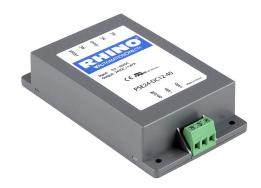
RHINO DC to DC converter, 9.5-36 VDC input, 24 VDC output, 1.67A, 40W, plastic housing, encapsulated, chassis mount, screw terminal.
