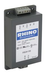
RHINO PSE series switching power supply, 24 VDC @ 1.25A/30W, 120/240 (47-440 Hz) VAC or 120-370 VDC nominal input, 1-phase, encapsulated, plastic resin and fiberglass housing, chassis mount, screw terminals.
