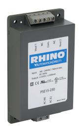
RHINO PSE series switching power supply, +15 VDC @ 1A/30W and -15 VDC @ 1A/30W, 120/240 (47-440 Hz) VAC or 120-370 VDC nominal input, 1-phase, encapsulated, plastic resin and fiberglass housing, chassis mount, screw terminals.
