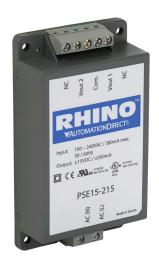
RHINO PSE series switching power supply, +15 VDC @ 0.5A/15W and -15 VDC @ 0.5A/15W, 120/240 (47-440 Hz) VAC or 120-370 VDC nominal input, 1-phase, encapsulated, plastic resin and fiberglass housing, chassis mount, screw terminals.
