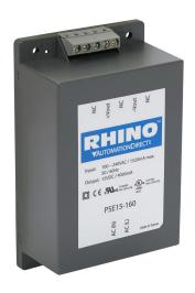
RHINO PSE series switching power supply, 15 VDC @ 4A/60W, 120/240 VAC nominal input, 1-phase, encapsulated, plastic resin and fiberglass housing, chassis mount, screw terminals.
