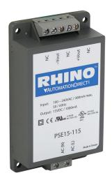
RHINO PSE series switching power supply, 15 VDC @ 1A/15W, 120/240 (47-440 Hz) VAC or 120-370 VDC nominal input, 1-phase, encapsulated, plastic resin and fiberglass housing, chassis mount, screw terminals.
