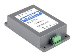
RHINO DC to DC converter, 18-75 VDC input, 12 VDC output, 3.33A, 40W, plastic housing, encapsulated, chassis mount, screw terminal.
