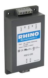
RHINO PSE series switching power supply, +12 VDC @ 1.3A/30W and -12 VDC @ 1.3A/30W, 120/240 (47-440 Hz) VAC or 120-370 VDC nominal input, 1-phase, encapsulated, plastic resin and fiberglass housing, chassis mount, screw terminals.
