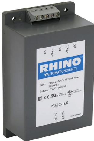
RHINO PSE series switching power supply, 12 VDC @ 5A/60W, 120/240 VAC nominal input, 1-phase, encapsulated, plastic resin and fiberglass housing, chassis mount, screw terminals.
