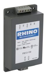
RHINO PSE series switching power supply, 12 VDC @ 2.5A/30W, 120/240 (47-440 Hz) VAC or 120-370 VDC nominal input, 1-phase, encapsulated, plastic resin and fiberglass housing, chassis mount, screw terminals.
