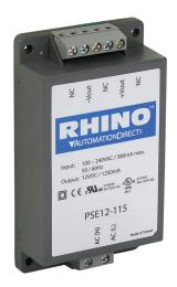
RHINO PSE series switching power supply, 12 VDC @ 1.25A/15W, 120/240 (47-440 Hz) VAC or 120-370 VDC nominal input, 1-phase, encapsulated, plastic resin and fiberglass housing, chassis mount, screw terminals.
