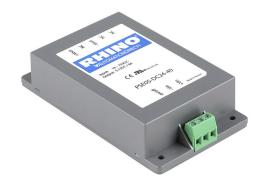
RHINO DC to DC converter, 18-75 VDC input, 5.1 VDC output, 8A, 40W, plastic housing, encapsulated, chassis mount, screw terminal.
