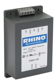
RHINO PSE series switching power supply, 5.1 VDC @ 10A/51W, 120/240 (47-440 Hz) VAC or 120-370 VDC nominal input, 1-phase, encapsulated, plastic resin and fiberglass housing, chassis mount, screw terminals.
