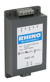
RHINO PSE series switching power supply, 5 VDC @ 6A/30W, 120/240 (47-440 Hz) VAC or 120-370 VDC nominal input, 1-phase, encapsulated, plastic resin and fiberglass housing, chassis mount, screw terminals.
