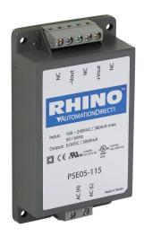
RHINO PSE series switching power supply, 5 VDC @ 3A/15W, 120/240 (47-440 Hz) VAC or 120-370 VDC nominal input, 1-phase, encapsulated, plastic resin and fiberglass housing, chassis mount, screw terminals.
