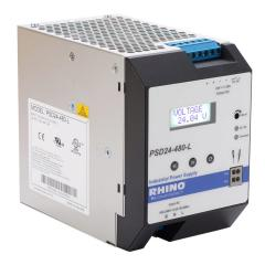
RHINO PRO PSD series switching power supply, 24 VDC @ 20A/480W (adjustable), 120/240 VAC or 110-300VDC nominal input, 1-phase, enclosed, aluminum housing, LCD display, 35mm DIN rail mount, screw terminals.
