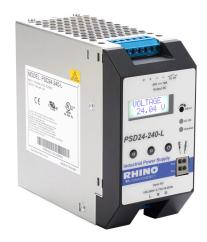
RHINO PRO PSD series switching power supply, 24 VDC @ 10A/240W (adjustable), 120/240 VAC or 110-300VDC nominal input, 1-phase, enclosed, aluminum housing, LCD display, 35mm DIN rail mount, screw terminals.
