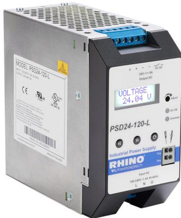
RHINO PRO PSD series switching power supply, 24 VDC @ 5A/120W (adjustable), 120/240 VAC or 110-300VDC nominal input, 1-phase, enclosed, aluminum housing, LCD display, 35mm DIN rail mount, screw terminals.
