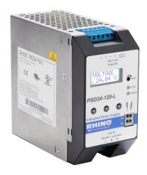
RHINO PRO PSD series switching power supply, 24 VDC @ 5A/120W (adjustable), 120/240 VAC or 110-300VDC nominal input, 1-phase, enclosed, aluminum housing, LCD display, 35mm DIN rail mount, screw terminals.
