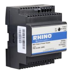
RHINO SELECT PSC series switching power supply, 24 VDC @ 2.5A/60W (adjustable), 120/240 VAC nominal input, 1-phase, enclosed, plastic housing, 35mm DIN rail mount, screw terminals, NEC Class 2.
