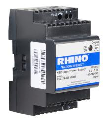
RHINO SELECT PSC series switching power supply, 24 VDC @ 1.25A/30W (adjustable), 120/240 VAC nominal input, 1-phase, enclosed, plastic housing, 35mm DIN rail mount, screw terminals, NEC Class 2.
